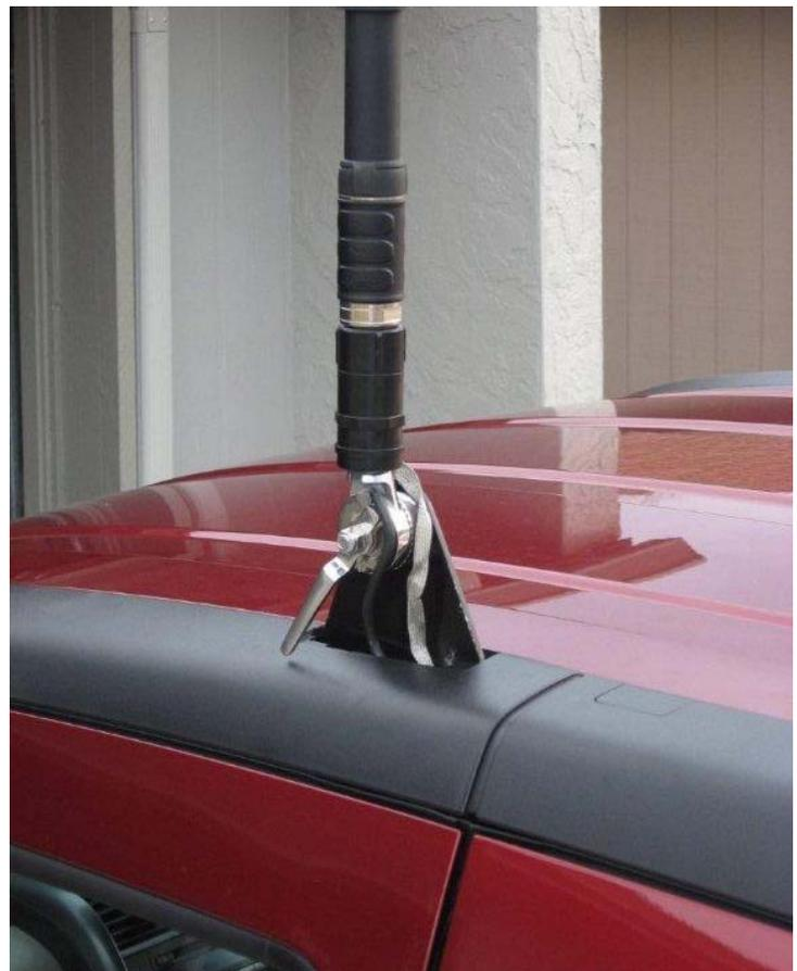
With a 90-degree movement of the handle, the ratchet teeth allow raising of the antenna. It will definitely handle the weight and wind and in about 15 seconds you're mobile. (Reprinted courtesy eHam.net)
